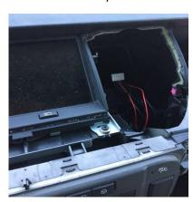
Connect the Climate control panel back with the 4 torx screws, be careful not to get any wires stuck, there is room for them behind climate control system
