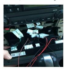
Connect then the 4 female connectors from cars wiring into male connectors from IPCU wiring loom
